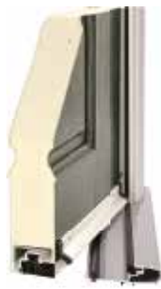
Mobility Access Threshold MDS80/2 (15mm) Distance from bottom of door leaf to bottom of threshold 18mm
